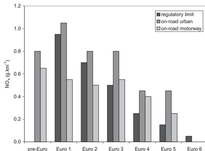
**Fig. 2.** NO<sub>x</sub> emission factors ( $\text{g km}^{-1}$ ) for diesel-fuelled passenger cars in accordance to EU testing cycles EU1 to EU6 and based on actual driving conditions at urban roads and motorways in the Netherlands.
