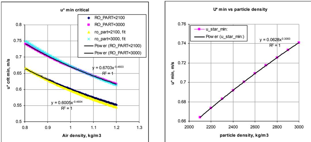
**Figure 6.** Dependence of minimal critical friction velocity on air and particle density (left) and on particle density (right)
