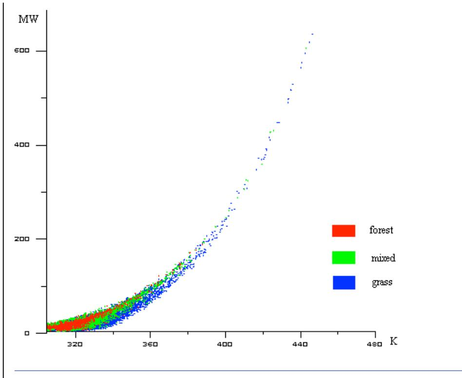
**Figure 1.** A relation between the fire intensity indicators. The brightness temperature, [K] from 21-st band of MODIS (horizontal axis) is related to FRP for the same fire pixel from MOD14 fire product [MW per pixel area] (vertical axis). Colours of the dots correspond to the land cover types (red – forest, green - mixed forest and grass, blue – grass only).
